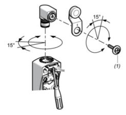
(1) Tightening torque (Min: 1) (Max: 1.5)
