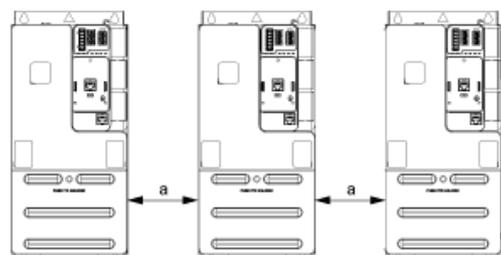
$a \geq 50$  mm (1.97 in.) from 50...60°C, no restriction below 50°C
