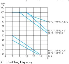
The derating curves for the drive nominal current (In) depend on the temperature, the switching frequency and the mounting type (A, B or C). For intermediate temperatures (45°C for example), interpolate between 2 curves.
