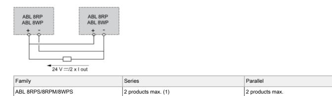
NOTE: Series or parallel connection is only recommended for products with identical references.
