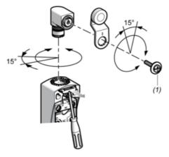
(1) Tightening torque (Min: 1) (Max: 1.5)
