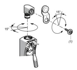
(1) Tightening torque (Min: 1) (Max: 1.5)
