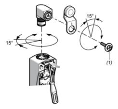
(1) Tightening torque (Min: 1) (Max: 1.5)
