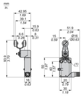
(1) 2 fixing holes  $\varnothing$  4.2 mm, counterbored  $\varnothing$  8 mm by 4 mm deep.
