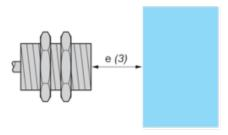
e (3) ≥ 7.5 mm/0.30 in. Mounted in a metal support
