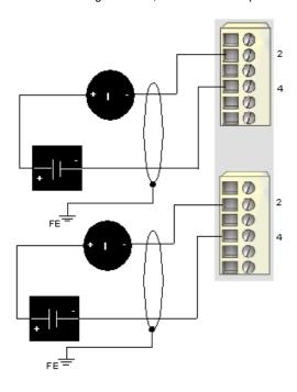
2 non-isolated analog actuators, 24 VDC supplied by the PDM
