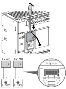
The (-) poles are connected internally.
