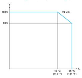
X: Ambient temperatureY: Input simultaneous ON ratio
