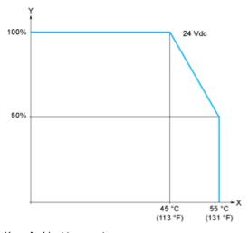
X: Ambient temperatureY: Input simultaneous ON ratio
