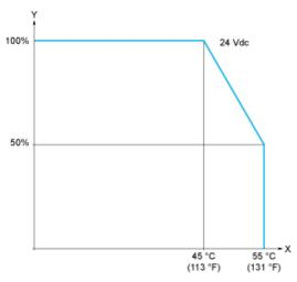
X: Ambient temperatureY: Output simultaneous ON ratio
