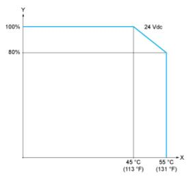
Ambient temperature Output simultaneous ON ratio
