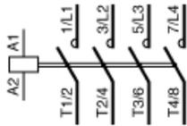
3-Pole Contactors: 3P + N/C
