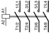
3-Pole Contactors: 3P + N/C
