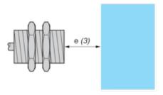
e (3) ≥ 7.5 mm/0.30 in. Mounted in a metal support
