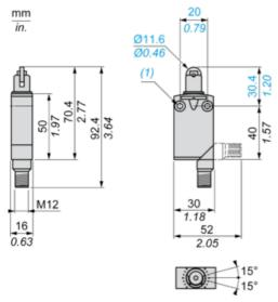
(1) 2 fixing holes  $\varnothing$  4.2 mm, counterbored  $\varnothing$  8 mm by 4 mm deep.
