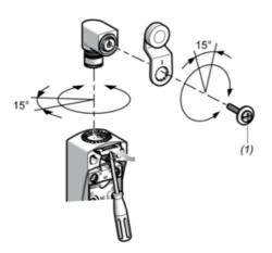
(1) Tightening torque (Min: 1) (Max: 1.5)
