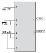
With External Device Monitoring (EDM) feedback loop
