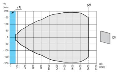
(X): Target distance (Y): Detection limit
