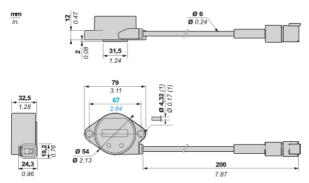
(1): The sensor is supplied with 2 stainless steel inserts and 2 silicone washers. M4 screws not provided.
